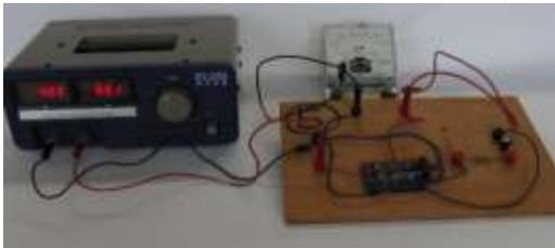
We set the voltage at 4volts and measured the value of the current until the condenser finished discharging electricity.
