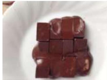
$$2.45 \times 10^9 (\text{Hz}) \times 1.10 \times 10^{-1} (\text{m}) \\ \approx 2.70 \times 10^8 (\text{m/s})$$
