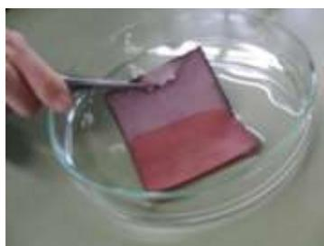
When we dropped pH4 on red test paper, it remained still. And at pH6 and over, it turned blue. We founded the test paper could distinguish pH4 between pH6.
