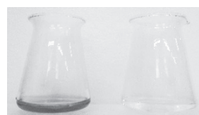
Figure.4 Color change after dripping \text{H}_2\text{SO}_4 (Left: Before dripping Right: After dripping)
